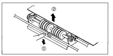
Take out the retard roller module in the optional "Roller Exchange Kit (KV-SS041)".
